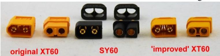
connector. XT60s comes in different colors, but this would have been the 1st non-blue EC3. Anyway, then I see it has printed SY60 on its side, and the back does not really look like EC3 – in short, it was not an EC3! It turns out to be a new connector, compatible with
