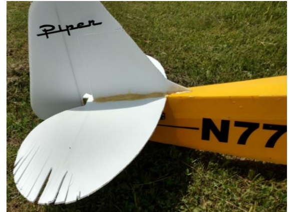
Prop strike on Brad's large cub (T. Eng)
