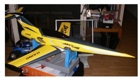
I bought a battery for it at the same time as I bought the plane. Once I had it assembled, I realized that even with the pushrods in place, it could be disassembled in a snap and would fit snug back into its foam tray and box, so that is where I will store it. Field assembly should be quick and fairly easy. And BTW, that pointy nose cone is held on with a magnet and is replaceable.
