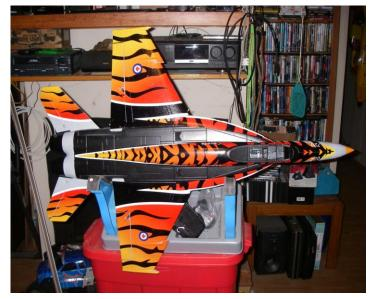
free shipping. This airplane has good points and bad points. The bad starts with the terrible manual which leaves the modeler a lot of questions. The wings plug into the fuse with a Carbon fiber wing tube and are held in place by magnets at the fuse-a not so good connection which leads people to use glue. What they don't mention in the manual is that there are several sharp pointed self threading screws and a plastic plate on the bottom of the wing directly in line
