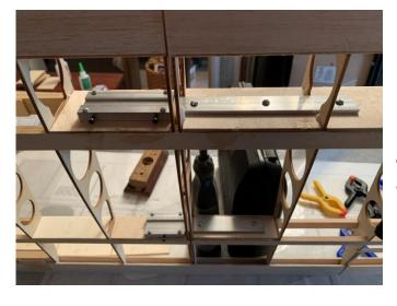
The aluminum channel and spar that connects the wings to the center section.
