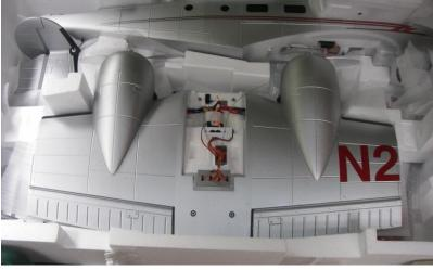
cerning the elevator. Read it and follow it. They include a gage for setting the elevator properly. Myself, I simply removed the elevator servo arm from the servo for the pushrod extension and I used the clevis at the elevator to adjust the deflection. I got it close with the tail assembly loose, then for the final adjustment I was able to spin the pushrod at the servo to adjust the clevis a couple more turns.
